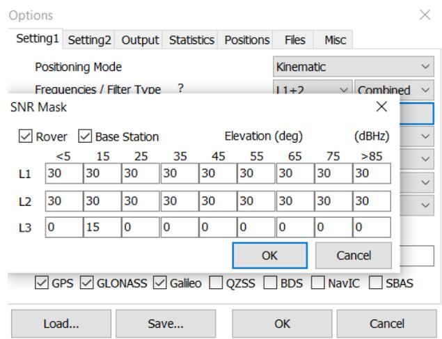
Figure 6. example for adjusting the SNR mask
