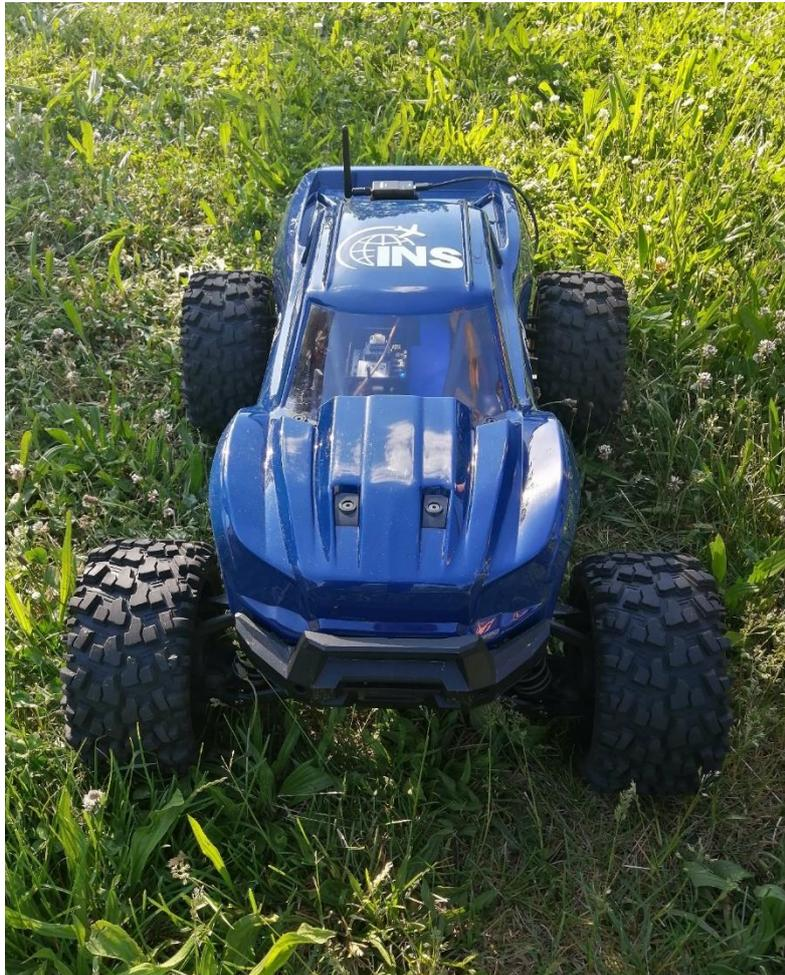
*Figure 1. Remote Controlled car used as rover*
