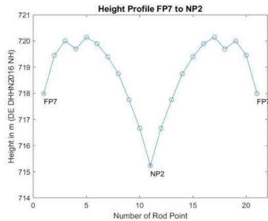
Figure 77: Loop of the New Line at the Airfield Hülben (selfmade in Google Earth Pro and MATLAB)
