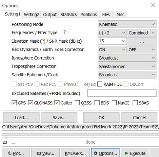
Figure 5. example for RTKlib settings
