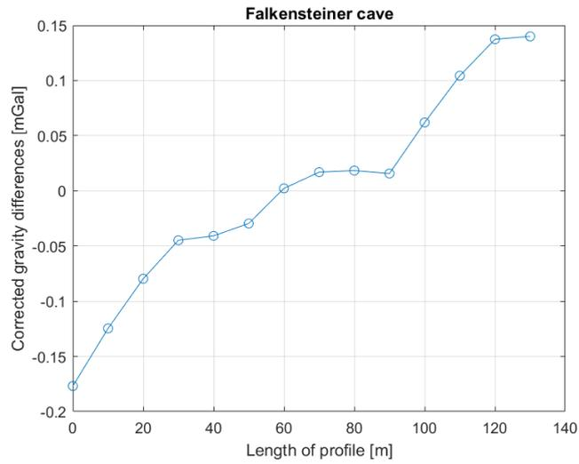
Figure 5: Gravity measurements Falkensteiner cave
