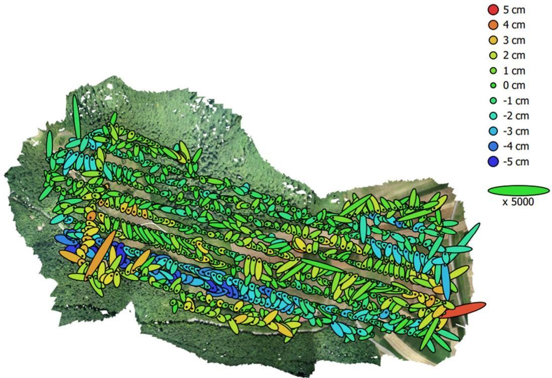
Z error is represented by ellipse color. X,Y errors are represented by ellipse shape. Estimated camera locations are marked with a black dot.
