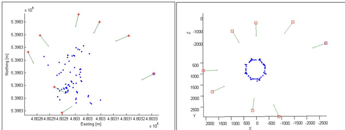
Figure 5. Forward intersection using the sensors data as exterior orientation parameters (left), Model created by relative orientation (right)
