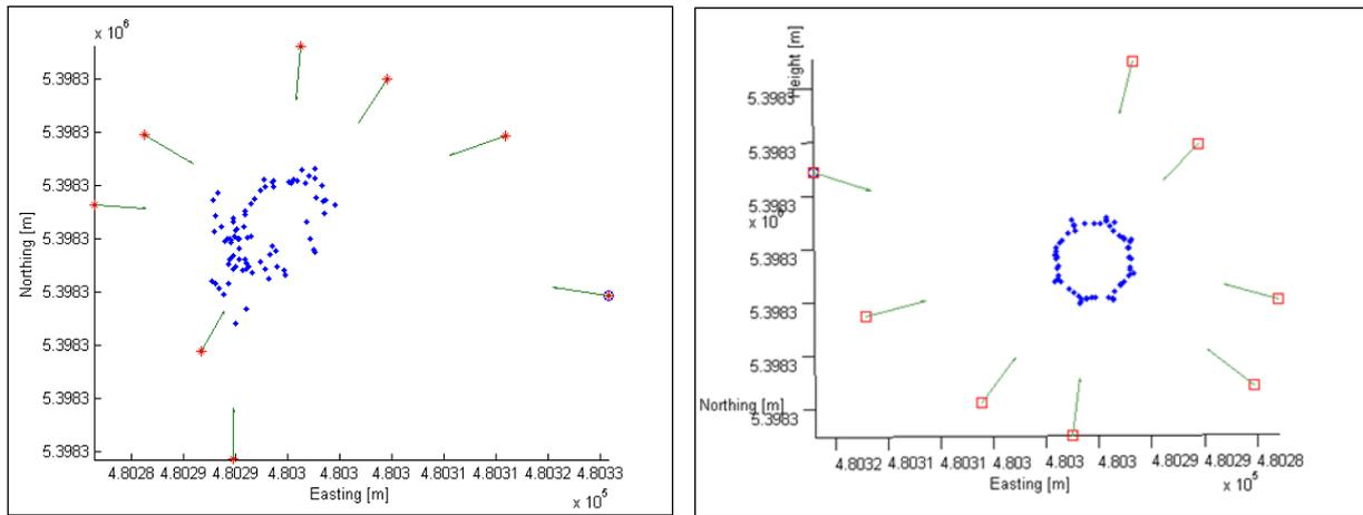
Figure 6. Forward intersection with raw sensor data but corrected azimuths (left), Results of the bundle block adjustment (right)
