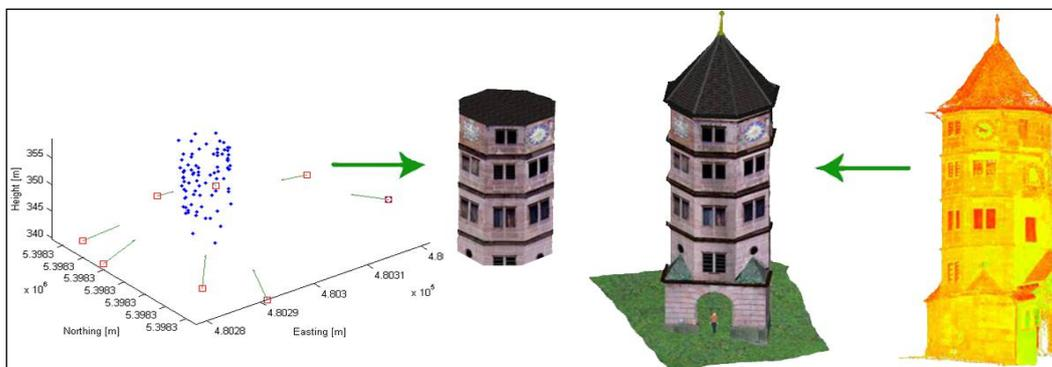
Figure 7. 3D models created by the described method (left) and terrestrial laser scanner (right)
