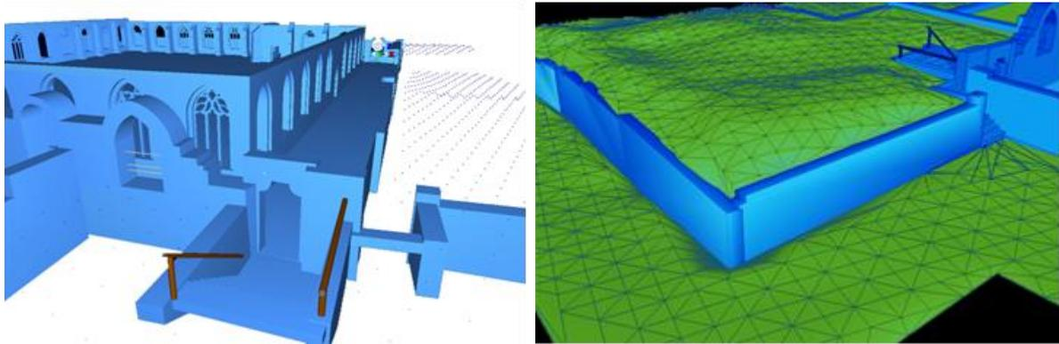
Figure 1. 3D modeling by shape fitting and triangulation
